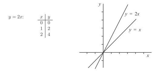
If we calculate the gradient of the line y = 2x using the first two sets of values in the table, we obtain
